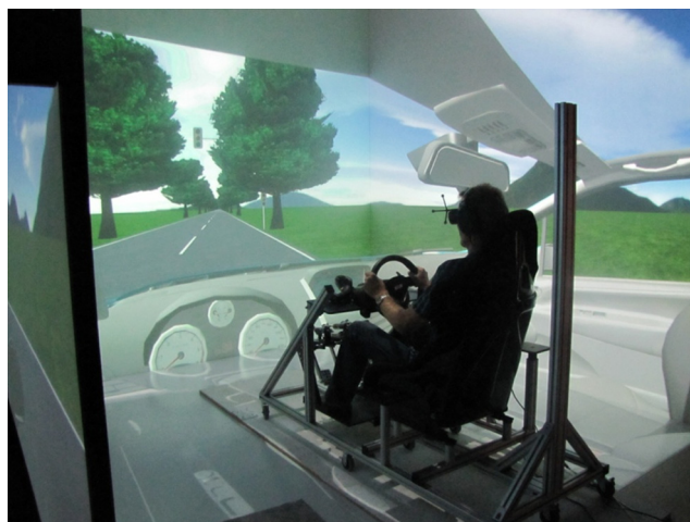
Fig. 1. Illustration of the main setup. A driving simulator was placed in a CAVE-like environment to provide realistic 3D visual stimuli to which different auditory stimuli were scaled and displayed to the drivers via earphones.
